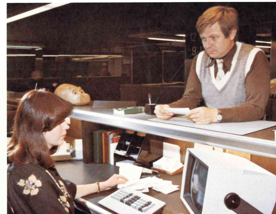
A modern banking terminal also includes a video display unit, as well as a printer and keyboard.
